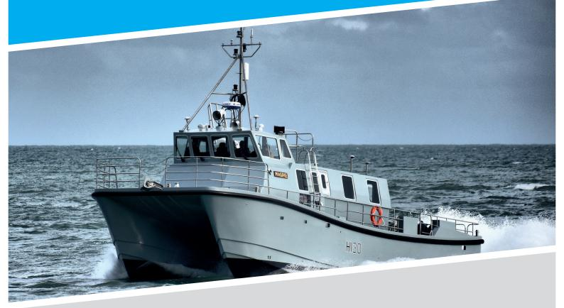
The 18m SEA Class Survey Motor Launch is the largest variant of the SEA Class range. Renowned for its sea keeping capability, the craft offers AEUK's modular and fully integrated capability for hydrographic survey. The craft is equipped with Single and Multi-beam Echo Sounders, motion reference equipment, as well as the S2094 towed side scan sonar system.
